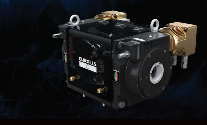
These cassettes work in association with **Boba25 control system**. Utilizing a **laser measurer** positioned at the machine's exit and performing **16,000 checks** per second, it keeps the wire's **weight and mass consistent**, working on the regulation of the rolls and the wire diameter.
